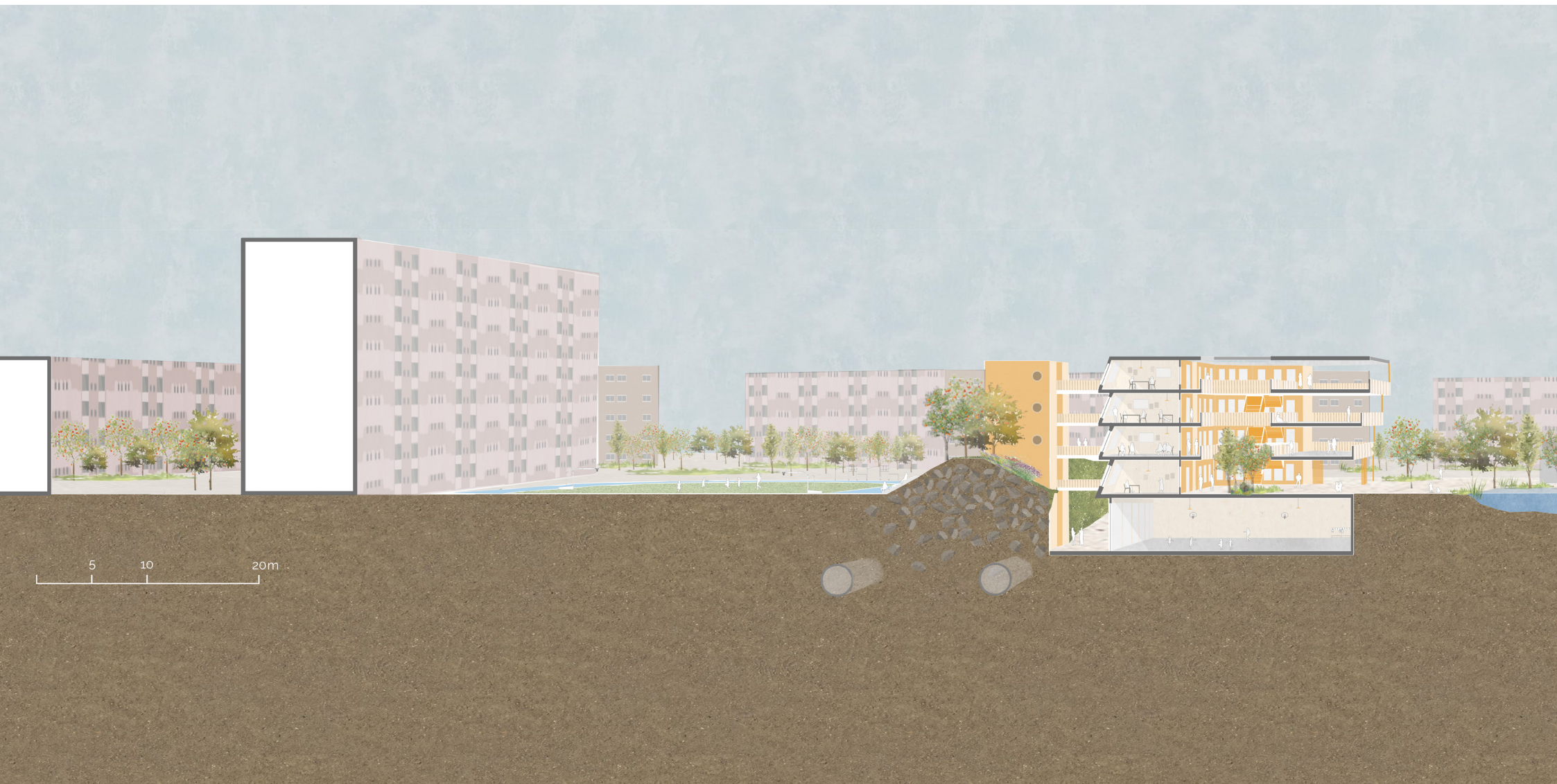
Heat store and earth cooling tubes
